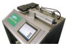
IAI devised a precision power to measure energy efficiency. Both the air cylinder and ROBO Cylinder were tested with identical variables. Variables included dwell time, cost of electricity, cost of compressed air, speed, payload, stroke, ambient temp and
