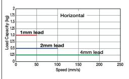
(1) The load capacity is based on operation at an acceleration of 0.2G.
